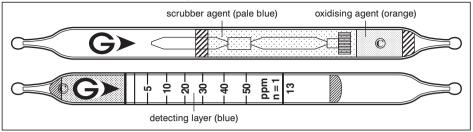
When used, these tubes are to be connected.
